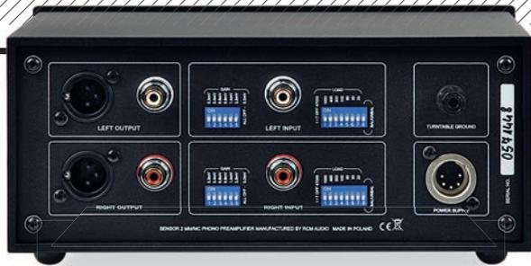
LEFT: RCA input may be rigged for balanced input alongside eight loading options and seven gain settings
